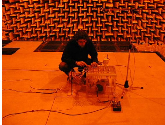
Fig. 6. Testing set-up in the anechoic chamber for the measurement of the sound power radiated by the smart panel when excited by the loudspeaker in the Plexiglas box or by the shaker mounted on the panel.
